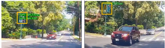
Fig. 1: Two video frames showing the same traffic light instance several seconds apart. A distinct object query is defined by having these two boxes only count as one result.
